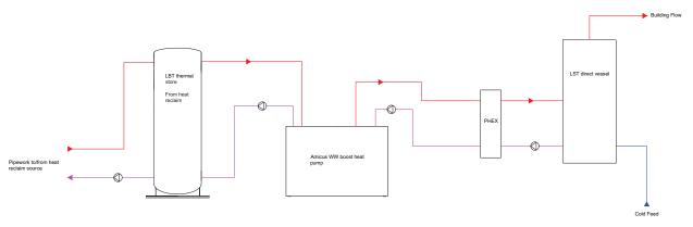
Amicus Boost heat pump with heat recovery/reclaim to provide hot water
